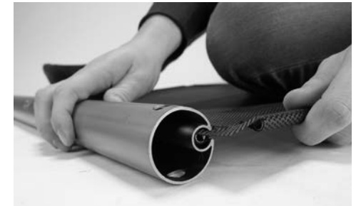
Abb. 6.5.4. Guide the tube along the length of the net
