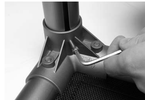
Abb. 6.9.2. Tighten the screw of the legs
