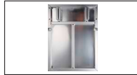
Fig. 5.9.1. Underside of the DogBus. The two insertion points are clearly visible in the upper part of the image.
