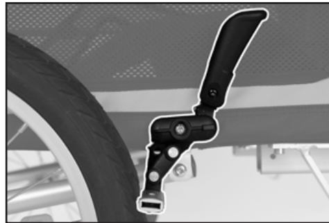
Fig. 5.5.1. Parking Brake Engaged. DogBus View – Right Side in Direction of Travel
